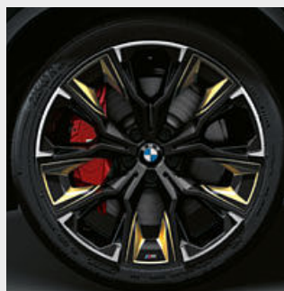
□ 20" M aerodynamic wheels 920 M Multicolour with Gold accent and run-flat tyres, gloss-lathed, wheel size 8J x 20 with 225/40 R20 tyres.4,6,*
